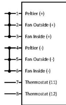
Bridged terminals are equipped with Wago 231-902 bridges from the factory & must be customized by the customer. The maximum wire diameter is 1,5 mm<sup>2</sup> when bridged and 2.5 mm<sup>2</sup> without bridge.
