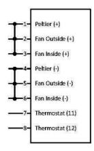
Bridged termianls are equipped with Wago 231-902 brigdges from the factory & must be customized by the customer. The maximum wire diameter is 1,5 mm<sup>2</sup> when bridged and 2.5 mm<sup>2</sup> without bridge.
