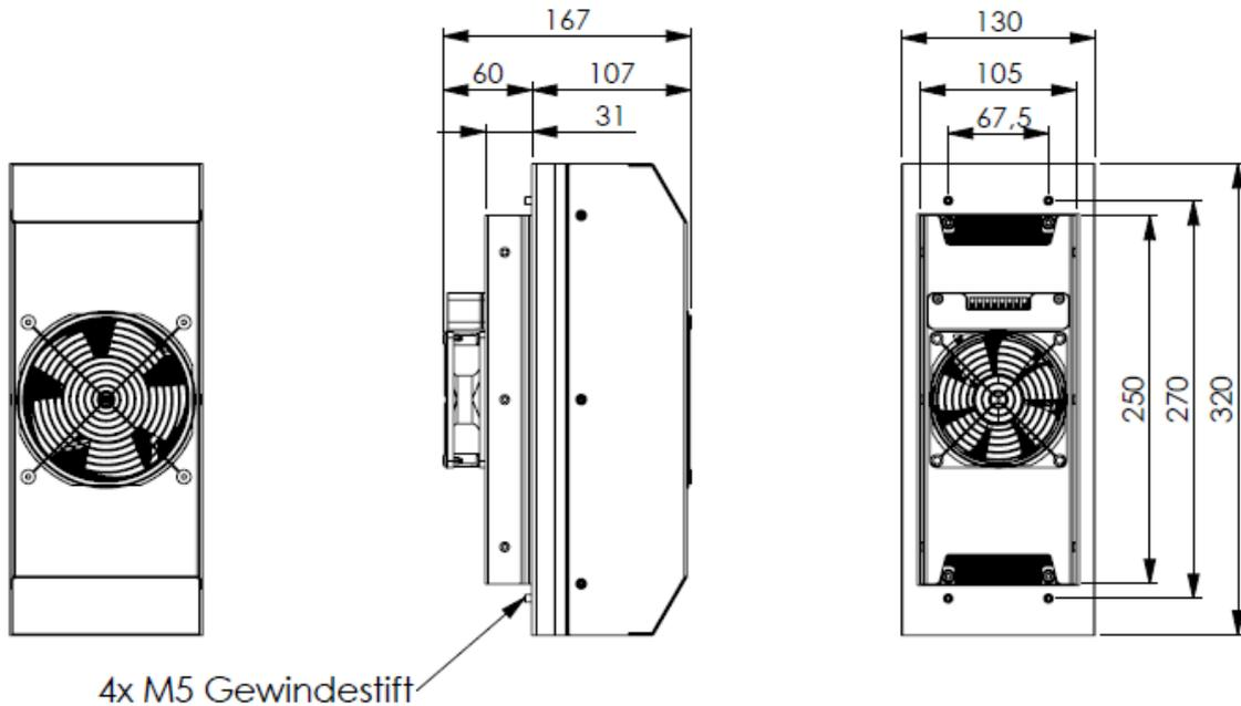
**PROTEMP 120 M | AA-120M-24-NN4-XXX-DNPT****5** ABMESSUNGEN
